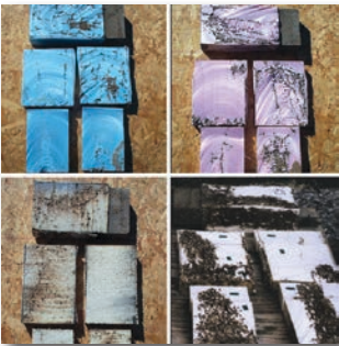
Termite-Damaged Untreated Foams
