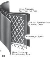
A layer of polyester scrim reinforcement placed between these plies greatly enhances tear resistance and increases service life. DURA+SKRIM® R20WWK is reinforced with a high strength scrim reinforcement laid in a diagonal pattern spaced 3/8" apart for uniform tear resistance in both machine and transverse directions with an additional machine direction scrim every 3" across the width for increased stability.
