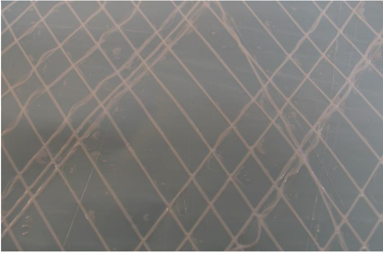
Inconsistency in the competitor reinforcing threads
