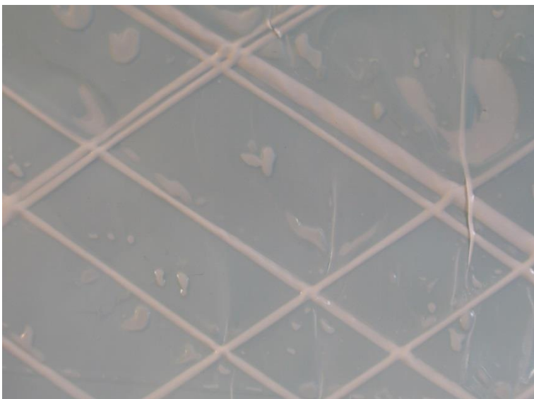
The competitor poly has delamination issues
