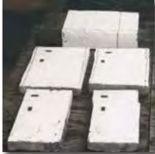
Bora-Foam Shows No Termite Damage
